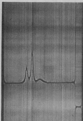
Figure 2. An example of the patterns of polymerization products of sample No. S-20: solvent, cyclohexane; 35 °C; concentration, 0.55%; 58780 rpm.
